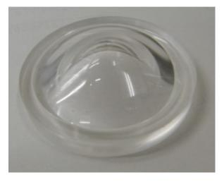
Fig. 11 Photograph of the actual turned aspherical lens.
