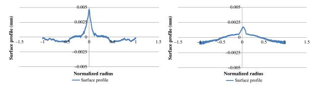
Fig. 12 Measured deviation of the turned lens from the designed shape.
