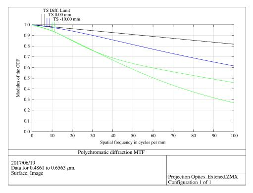
Fig. 10 MTF curve for the design described in Table 4 (blue line: on-axis, green-line: marginal tangential and radial).
