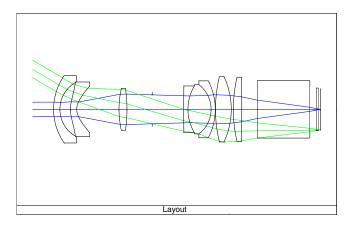
Fig. 9 Optical configuration of the lens represented in Table 4.
