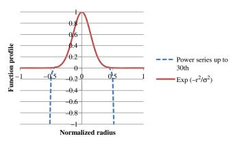
**Fig. 5** Comparison of the power series up to 30th with the normal distribution function for  $\sigma = 0.2$ .
