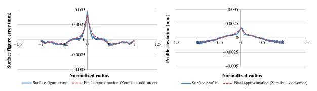
Fig. 14 Measured figure errors and the final approximation shapes.
