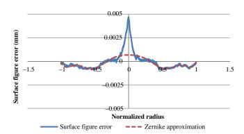
Fig. 1 An example of surface figure error and its Zernike approximation.
