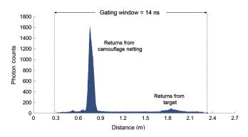
Fig. 3 Example of an aggregated timing histogram of a measurement of a target placed ~1 m behind camouflage netting. In this aggregated histogram, data from all 12800 pixels in the image are summed and displayed in this single histogram. In the figure, the larger peak consists of the returns from the camouflage netting and the smaller peak represents the returns from the target. The zero point in the depth axis is chosen arbitrarily, the camouflage netting was ~230 m from the transceiver.
