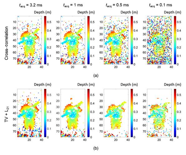
**Fig. 9** Depth profiles of the target (actor holding a wooden plank) standing 1 m behind the camouflage netting. The depth reconstruction is for four different per-pixel acquisition times of 3.2, 1, 0.5, and 0.1 ms (shown left to right). (a) The pixelwise cross correlation algorithm used for time-gated data corresponding to 4 ns and (b) the new TV +  $L_{21}$  algorithm for the same time-gated data used in (a). This figure shows downsampled images of  $40 \times 80$  pixels.
