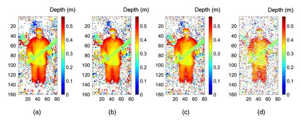
**Fig. 6** Depth profiles of an unobstructed target (an actor with a wooden plank held across the chest) at a range of 230 m. The pixel format was  $80 \times 160$  ( $X \times Y$ ). Depth profiles were reconstructed from data with reduced acquisition time: (a) 3.2 ms per pixel, (b) 1.0 ms per pixel, (c) 0.5 ms per pixel, and (d) 0.1 ms per pixel.
