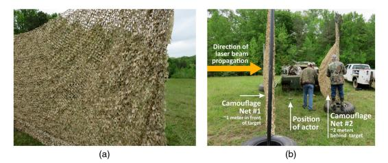
**Fig. 4** (a) Front view photograph of the double layer of commercially available camouflage net which was located 1 m in front of the target position. (b) Side view of the setup showing both a double layer of camouflage in front of the target and a single layer behind the target.
