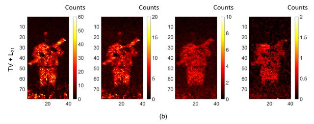
**Fig. 10** Intensity profiles of the target (actor holding a wooden plank) standing 1 m behind the camouflage netting. The intensity reconstruction is for four different per-pixel acquisition times of 3.2, 1, 0.5, and 0.1 ms (shown left to right). (a) The pixelwise cross correlation algorithm used for time-gated data corresponding to 4 ns and (b) the new  $TV + L_{21}$  algorithm for the same time-gated data. This figure shows downsampled images of  $40 \times 80$  pixels.
