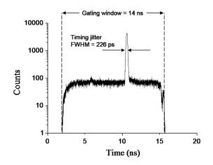
**Fig. 2** Instrumental timing response taken from a uniform, scattering surface located in the same nominal plane as the target. The overall timing jitter (226 ps FWHM) of the system and the detector gating window of 14 ns duration are shown in the figure. An arbitrary zero was chosen for the displayed time-scale.
