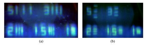
Fig. 10 Resolutions of reconstructed images (a) horizontal and (b) vertical resolutions.
