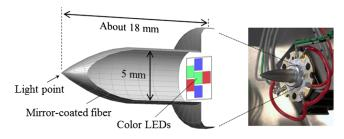
Fig. 6 Photo and details of full-color point light source unit with mirrorcoated fiber.
