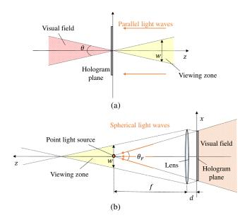
Fig. 1 Outlines the optical reconstruction arrangements (a) conventional and (b) FTOS.
