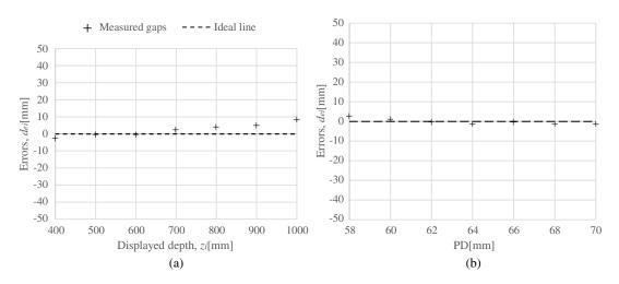
Fig. 13 Results of the vergence-value correction (a) measured errors  $d_{ei}$  related to the vergence and (b) related to PDs.
