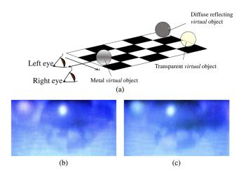
Fig. 8 Parallax of the holographic HMD (a) schematic diagram and (b) view from left and (c) view from right.
