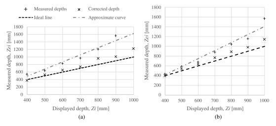
Fig. 12 Results of depth correction (a) measured depths and corrected depths of left optical unit, (b) right unit.
