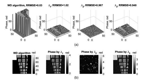
**Fig. 6** USAF phase reconstructions RRMSE = 0.030 for SNR = 3.8 dB ( $N_{\text{photon}} = 0.75$ ), (a) 3-D surfaces and (b) 2-D absolute phases. From left to right: the WD algorithm, and the single wavelength reconstructions for  $\lambda_1$ ,  $\lambda_2$ , and  $\lambda_3$ , respectively.
