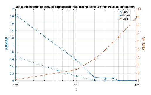
**Fig. 3** RRMSE and SNR as function of the parameter  $\chi$  of the Poissonian distribution: solid triangles and dashed diamonds curves (blue in color images) show RRMSE for the Gaussian and USAF objects, respectively (left *y*-axis); solid circle curve (orange) shows SNR of the observations (right *y*-axis).
