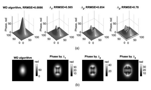
**Fig. 5** Gaussian phase reconstructions RRMSE = 0.0086 for SNR = 6.5 dB ( $N_{photon}$  = 1.87), (a) 3-D surfaces and (b) 2-D absolute phases. From left to right: the WD algorithm, and the single wavelength reconstructions for  $\lambda_1$ ,  $\lambda_2$ , and  $\lambda_3$ , respectively.
