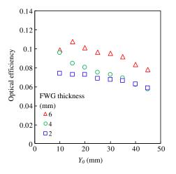
**Fig. 9** Optical efficiency for collecting light at the bottom edge of an FWG. The excitation spot was moved on the y axis in the coordinate system defined in Fig. 1(a). As the spot moves away from the edge, the efficiency decreases.
