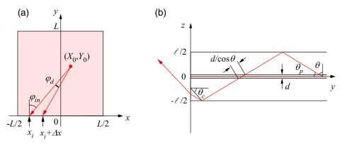
**Fig. 1** Trajectories of the light from an isotropic point source placed at a single spot in a rectangular parallelepiped waveguide. The probabilities of the light reaching and exiting the waveguide in the *xz* plane are expressed as a function of the coordinate of the point source: (a) top view and (b) cross section.
