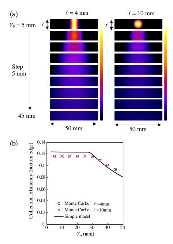
**Fig. 4** Radiance distributions obtained by a 3-D Monte Carlo simulation for the monochromatic light exiting the bottom edge. The point source is moved on the y axis with increments of 5 mm: (a) comparison of the distributions for a 4-mm-thick plate and those for a 10-mm-thick plate and (b) the ECFs obtained by the Monte Carlo simulation and the simple analytical model are compared.
