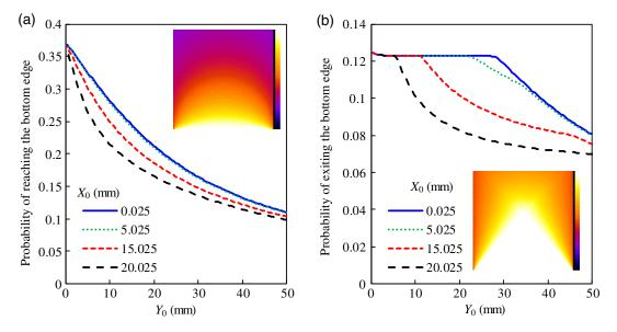
Fig. 3 ECF for the example in Fig. 2: (a) the ECF for the light reaching the bottom edge and (b) the ECF for the light exiting the waveguide from its bottom edge.
