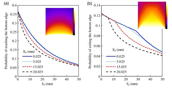
**Fig. 5** ECFs for a weakly absorbing case ( $\mu_0 = 0.01 \text{ mm}^{-1}$ ): (a) the ECF for the light reaching the bottom edge and (b) the ECF for the light exiting the waveguide from its bottom edge.
