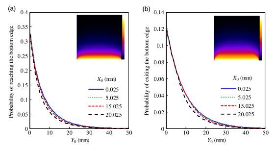
**Fig. 6** ECFs for a strongly absorbing case ( $\mu_0 = 0.1 \text{ mm}^{-1}$ ): (a) the ECF for the light reaching the bottom edge and (b) the ECF for the light exiting the waveguide from its bottom edge.
