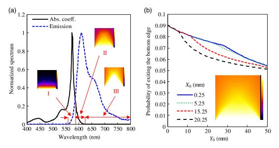
**Fig. 7** A TECF is roughly calculated by dividing the emission spectrum into three wavelength ranges and weighting a representative ECF in each range by the proportion of the photons within its range. (a) Normalized absorption coefficient and emission spectrum of Lumogen F Red 305. (b) The inset image is the resultant TECF and the curves are the TECFs along the specified *x* coordinates ( $X_0$ ).
