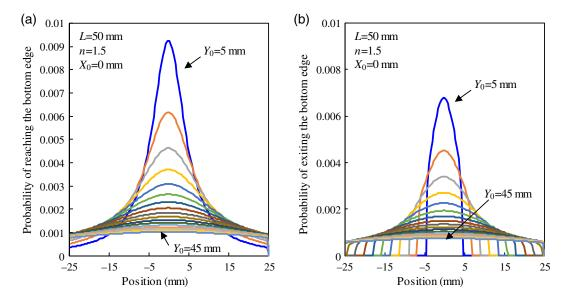
**Fig. 2** Numerical example for the probability of the light (a) reaching and (b) exiting the bottom edge surface. The isotropic point source is assumed to be at  $(X_0, Y_0)$  in a 50 mm × 50 mm FWG with refractive index of 1.5.
