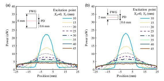
**Fig. 8** Intensity distributions measured by the PD array placed in the vicinity of the bottom edge: (a) 6-mm-thick FWG and (b) 2-mm-thick FWG. The incident power was 121  $\mu$ W for the 6-mm-thick FWG and 49.8  $\mu$ W for the 2-mm-thick FWG. The inset in each graph shows the cross section of a PD facing the edge surface of the FWG.
