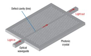
**Fig. 5** A 2-D PhC waveguide adapted from Ref. 30. The top and bottom milled areas form a PhC with a photonic bandgap. Light is confined to defects which, here, is the region absent of holes, which forms the central waveguide. Introducing analytes near the PhC changes the RI and the cutoff frequencies of the bandgap.
