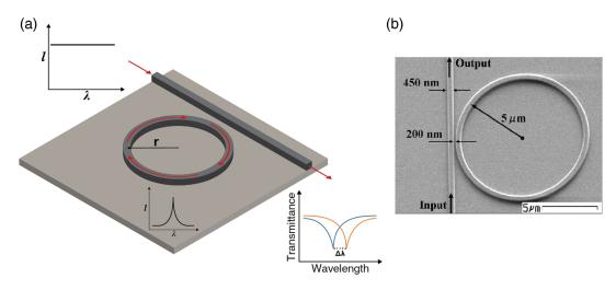
**Fig. 4** Ring-resonator sensor. (a) Schematic of a ring-resonator sensor. The linear waveguide provides input light to the loop waveguide at the coupling zone and captures output light from the loop for measurement. The presence of analyte will shift the resonance wavelength within the loop, which is detected in the output spectra, adapted from Ref. 10. (b) Micrograph of a fabricated ring resonator, adapted from Ref. 22.
