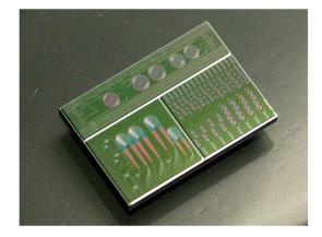
Fig. 6 PIC sensor device with integrated photonics and electronics manufactured by the AIM Photonics teams.
