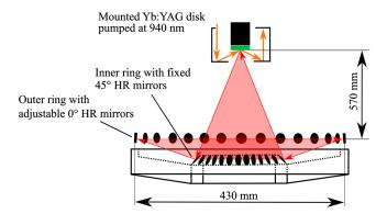
**Fig. 6** Concept of the compact multipass amplifier. The beam path of the pump and seed beam is indicated by orange and red arrows, respectively. The HR mirrors (AOI 45 deg) mounted in the inner ring unfold the solid angle onto the outer ring, where HR mirrors (AOI 0 deg) are mounted in adjustable mirror holders to fold the beam multiple times over the thin-disk.
