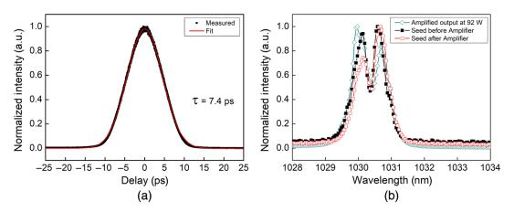
**Fig. 11** (a) Autocorrelation trace and fit at 92 W of average output power in configuration V. From the autocorrelation trace the pulse duration was determined to be 7.4 ps (FWHM, assuming a Gaussian temporal shape). (b) Normalized spectra of the unamplified seed laser before and after the amplifier and the amplified beam at 92 W of output power in configuration V.
