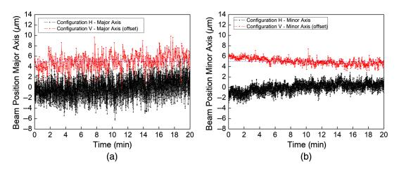
**Fig. 14** Beam positions on a camera chip in dependence of the time for the major (a) and minor (b) axis of the distributions shown in Fig. 13. For improved illustration, an offset of 5  $\mu$ m was added to the data of configuration *V* in both plots.
