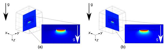
**Fig. 4** Distribution of the temperature of the ambient air in the (a) y-z and (b) x-z sectional plane for a disk mounted in configuration V.
