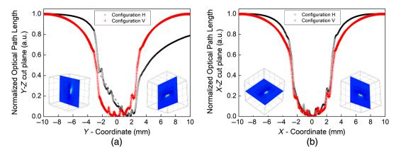
**Fig. 5** (a) Calculated distribution of the OPL in the *y*-*z* (a) and the *x*-*z* (b) plane. The pumped area is centered at x = y = 0 and extends to  $\pm 2.4$  mm. The insets indicate the corresponding planes, as shown in Figs. 2 and 4.
