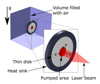
**Fig. 1** Schematic illustration of the thin disk in its conventional orientation facing in horizontal direction (configuration *H*). The arrow marked "g" indicates the direction of gravitational acceleration, which determines the direction of convection. The surface normal of the laser crystal coincides with the propagation axis of the laser beam (*z* axis).
