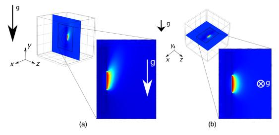
**Fig. 2** Distribution of the temperature of the ambient air (a) in the vertical (y-z) and (b) in the horizontal (x-z) sectional plane for configuration *H*.
