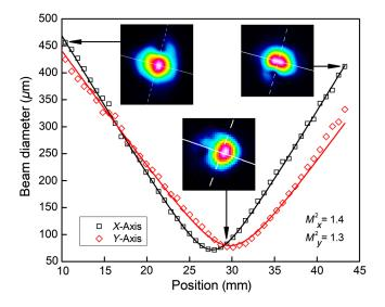
Fig. 10 Beam quality measurement at an output power of 92 W in configuration V. The insets depict the intensity distributions of the amplified beam.
