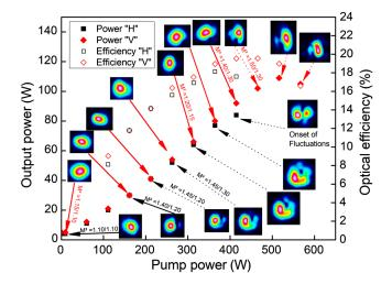
**Fig. 8** Output power and optical efficiency (seed power subtracted) of the amplifier in configuration H (black) and V (red). The insets show the far-field intensity distributions of the amplified laser beam at the corresponding pump power. Solid arrow lines indicate  $M^2 \le 1.4$ , while dashed arrow lines indicate  $M^2 > 1.4$  in at least one transverse axis of the caustic.
