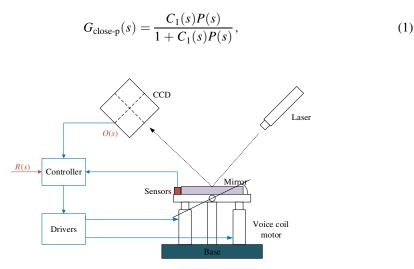
Fig. 1 Configuration of an image-based tracking control system for tip-tilt mirror.
