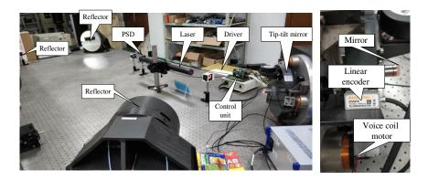
Fig. 5 Configuration of experimental platform: (a) global diagram and (b) local diagram of tip-tilt mirror.
