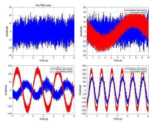
**Fig. 9** Error comparisons between the position-rate control and the two-position control: (a) PSD noise, (b) error comparison at 0.1 Hz, (c) error comparison at 0.5 Hz, and (d) error comparison at 1 Hz.
