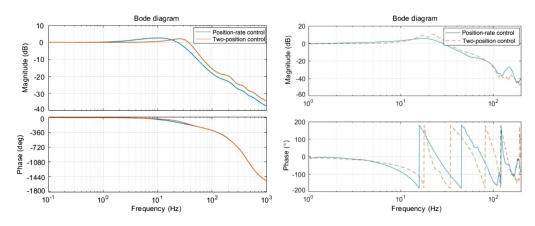
Fig. 6 Tracking control closed-loop responses of the tip-tilt mirror system: (a) simulation and (b) experiment.
