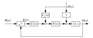
Fig. 10 Functional block diagrams with disturbance feedforward control.
