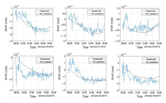
**Fig. 8** Apparent shift of the mountain peak as a function of local time for the JER experiment for January 20 to 25, 2019, daytime: time-lapse image measurement (blue) and the ML model prediction (black).
