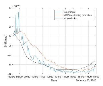
**Fig. 6** Apparent shift of the mountain peak as a function of local time for the WSMR experiment on February 2018: time-lapse image measurement (blue), NWP + ray-tracing prediction (red), and the ML model prediction (black).
