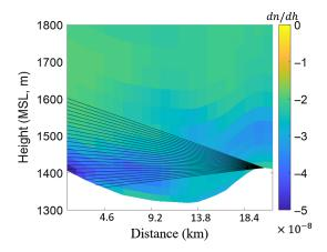
**Fig. 5** Example refractive index gradient results from NWP for the JER experiment on July 18, 2018, at 7:10 am MDT. Example ray paths are shown between the camera (left) and the target feature (right), which is a lower part the mountain ridge.
