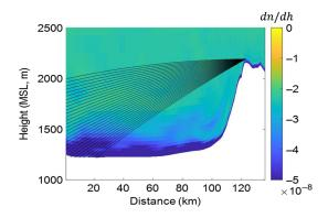
**Fig. 4** Example refractive index gradient results from NWP for the WSMR experiment on February 5, 2018, at 7:50 am MST. The white area is the ground. The time-lapse camera is located in the basin on the left and a peak in the Oscura Mountains is on the right. Example ray-tracing paths are shown between the target position on the peak and the area near the camera.
