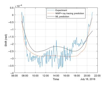
**Fig. 7** Apparent shift of the lower mountain ridge as a function of local time for the JER experiment on July 18, 2018: time-lapse image measurement (blue), NWP + ray-tracing prediction (red). and the ML model prediction (black).
