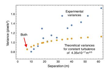
**Fig. 7** Differential tilt-variances computed for all pairs of sources for experimental data (blue) and a modeled constant turbulence level of  $4.35 \times 10^{-17}$  m<sup>-2/3</sup> (gold). Theoretical turbulence level chosen to overlap with experiment at point labeled "both."
