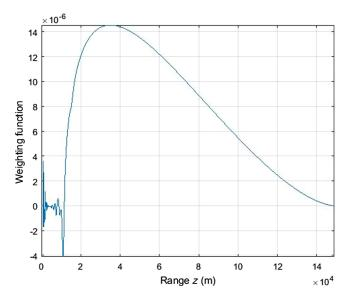
Fig. 3 Weighting function synthesized from linear combination of camera motion invariant weighting functions.
