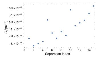
Fig. 8 Estimated turbulence for each source pair separation.
