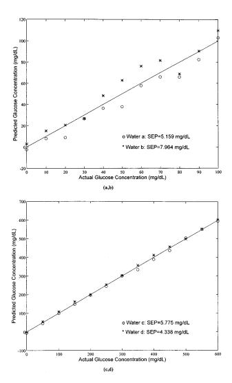
**Fig. 2** Glucose-doped water data showing true prediction of the glucose concentration of one data set based on a linear regression model using the other data set for both (a,b) the low concentration and (c,d) high concentration ranges. The data sets were taken with the digitally controlled benchtop polarimeter system using a 1 cm test cell. The line is shown for reference as the theoretical perfect fit.
