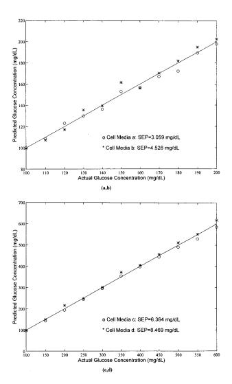
**Fig. 3** Glucose-doped bovine serum-based cell culture medium showing true prediction of the glucose concentration of one data set based on a linear regression model using the other data set for both (a,b) the low concentration and (c,d) high concentration ranges. The data sets were taken with the digitally controlled benchtop polarimeter system using a 1 cm test cell. The line is shown for reference as the theoretical perfect fit.
