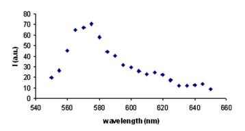
**Fig. 2** Spectral analysis of the red Cy3 dye. The figure shows the spectral analysis, elaborated from several spectral acquisitions within the 560- to 660-nm range, with a wavelength resolution of 5 nm, of the fluorescence intensity of the red Cy3 dye (exc. 543.5/em. 578 nm) (color online only).
