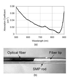
**Fig. 2** (a) Absorption coefficient of the SMP as a function of wavelength. Absorbance data was acquired using a Cary 300 spectrophotometer (Varian, Inc., Palo Alto, CA). (b) Microscope image of an SMP diffuser showing the optical fiber (125  $\mu$ m diameter including the polyimide coating) embedded in an SMP rod (300  $\mu$ m diameter). The polyimide coating was burned off of the optical fiber prior to cleaving the tip.
