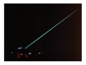
**Fig. 19** Copper vapor laser used as a laser guide star with a 1.5-m telescope at the Air Force Starfire test range in New Mexico. (Courtesy of Colin Webb)
