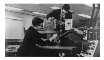
Fig. 3 Peter Sorokin (left) and Mirek Stevenson (right) adjust their cryogenically cooled uranium-CsF<sub>2</sub> laser at the IBM T. J. Watson Research Center. (Courtesy of IBM)
