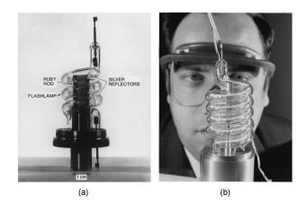
**Fig. 2** (a) Theodore Maiman's first laser, removed from aluminum cylinder used during operation, and (b) photo of Maiman behind a larger ruby laser, handed out at the Hughes press conference announcing the laser. The photographer insisted on posing Maiman with the larger laser, and initially many thought this was the first laser. (Courtesy of Kathleen Maiman)
