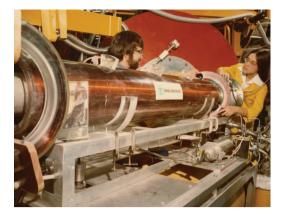
**Fig. 16** Gary Tisone (left) and A. Kay Hays (right) set up an electron-beam pumped ArF laser experiment at Sandia National Laboratories. (Courtesy Sandia National Labs)
