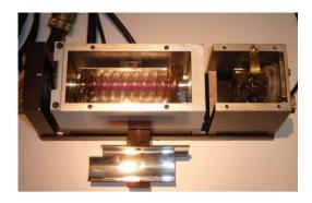
**Fig. 7** Korad's first commercial ruby laser, serial #001 of model RL-4KCS. The box at the right is a liquid Q switch. Comparison with Fig. 2(a) shows that Maiman's original design has been modified by using a longer flashlamp with more coils and a longer rod. (Courtesy of anonymous reviewer)
