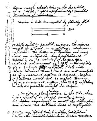
Fig. 1 First page of Gordon Gould's November 1957 notebook shows his sketch of a Fabry-Pérot laser resonator and comments about resonator mirrors. (Courtesy of Gordon Gould)
