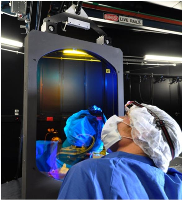
Fig. 10 Beamsplitter being craned into position.
