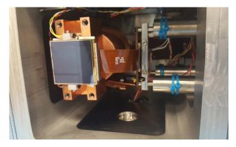
**Fig. 5** The WRXR camera chamber with H2RG (at image left) and SIDECAR<sup>TM</sup>, which is connected to the H2RG via the ribbon cable in the center of the chamber.
