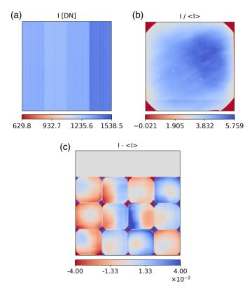
**Fig. 6** The calibration data used in the test run were recorded in the laboratory. (a) The dark field shows the characteristic sensor pattern: four distinct vertical stripes due to the four different readout channels. (b) The flat field used in the tests shows a gradient across the FOV, and a few dustgrains. (c) The  $4 \times 4$  demodulation matrix, **D**, depends on the FOV. To show this dependence in the plot, we subtract from each of the elements their spatial mean.
