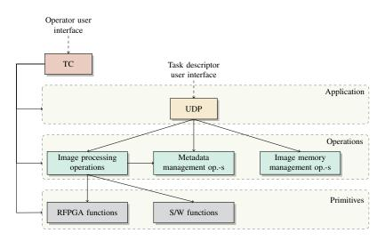
Fig. 3 The data processing software is organized on three layers. This organization facilitates information hiding, and the removal of responsibilities from the application developer (task descriptor).
