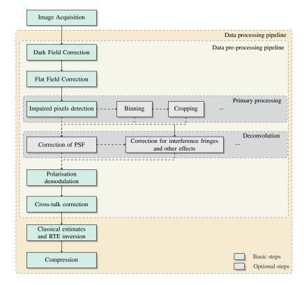
**Fig. 2** The on-board science data processing on SO/PHI follows the typical ground processing used for spectropolarimeters. It consists of mandatory (basic, shaded green in the figure) and optional steps (shaded light gray). Some of the optional steps will be used in specific science cases, for others we decide during instrument commissioning whether they are necessary.
