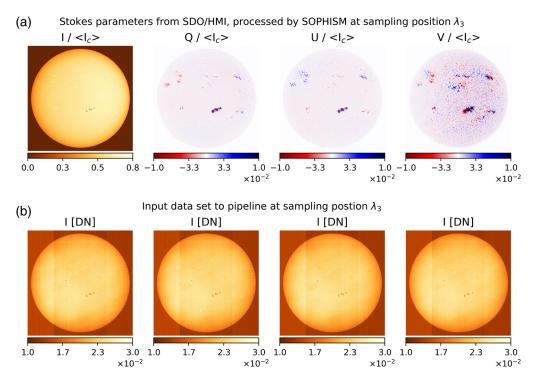
**Fig. 5** Test data set at the third wavelength sample. (a) The input to the pipeline are the Stokes images from SO/PHI Software siMulator (SOPHISM).<sup>37</sup> (b) The input images are obtained applying Eq. (5) and show similar light levels in all polarization states as a result of the modulation. The data also show the effect of the dark field (stripes) and the flat field (smudges and dust grains).
