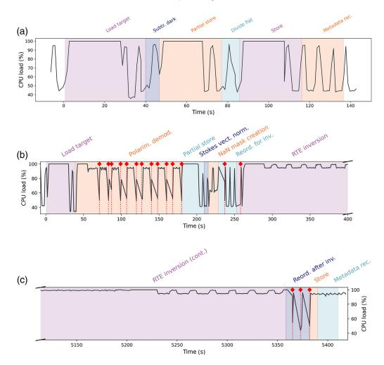
**Fig. 9** CPU load during the execution of the (a) image linear and (b, c) image parallel pipelines in nominal configuration. The colours show the execution of different pipeline blocks (see Fig. 4). The red dotted lines with diamonds indicate the times of RFPGA reconfigurations. During the polarimetric demodulation, there are 12 reconfigurations, which will be entirely removed in the future. The full pipeline takes little over 1.5 h to complete.
