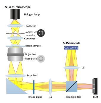
**Fig. 1** Spatial light interference microscopy (SLIM) optical setup. The phase is retrieved by shifting the phase of the scattered light with respect to that of the unscattered light by using a spatial light modulator (SLM) at the Fourier plane of lens L1. Four interferograms, correponding to four different SLM phase shifts, are obtained and used to compute the phase.<sup>17</sup>
