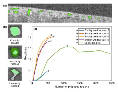
**Fig. 3** (a) Manually labeled tubule lumens (green regions), (b) overlaps between proposed regions (white) and manually labeled true regions (green), and (c) recall rate versus number of proposed regions for different algorithms.
