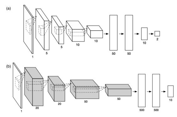
**Fig. 6** (a) An end-to-end trained small ConvNet and (b) LeNet with only the fully connected layer being trained while the rest (gray) of the layers inherited from the pretrained network trained on MNIST database.
