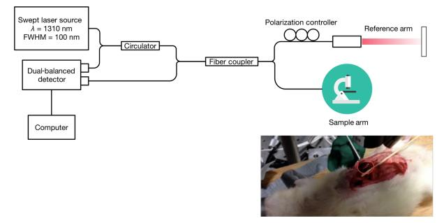
**Fig. 1** The schematic diagram of the custom-built OCT system used in this study. Inset image shows the abdominal cavity of a Munich-Wistar rat opened through a midline incision and the exposed left kidney for OCT imaging.
