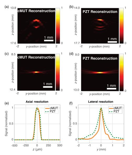
**Fig. 5** Comparison of the optoacoustic images acquired with the cMUT and PZT, showing significantly stronger limited-view artifacts for the latter. In (a) and (b) images of an 800- $\mu$ m diameter tube filled with India ink solution are shown. In (c) and (d) images of a 100  $\mu$ m absorbing suture are shown. (e, f) The axial and lateral resolution of the reconstructed suture images in (c) and (d).
