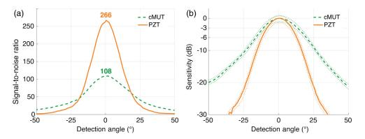
Fig. 3 Amplitude-based directivity comparison of the cMUT (dashed green) and PZT transducers (solid orange). (a) SNR as a function of the incidence angle for both transducers. (b) Normalized sensitivity plots showing a strongly favorable sensitivity of the cMUT for larger angles. Solid and dashed lines in (b) represent the smoothed mean, and dotted lines show the confidence interval with 1 standard deviation.
