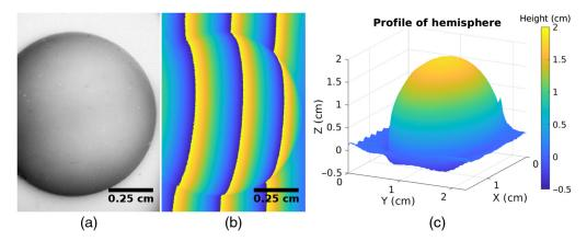
**Fig. 7** (a) Raw intensity image of a 1.75-cm-diameter hemispheric phantom showing how the intensity changes as a function of height. (b) Wrapped phase image of the same phantom. The effect of height can be clearly seen by the curve of the phase isolines. (c) Three-dimensional rendering of the object's profile following phase unwrapping and calibration of panel (b).
