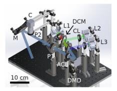
**Fig. 2** CAD rendering of the openSFDI system with the light paths for the three wavelengths. L, light-emitting diode; CL, collimating lens (only one of three labeled); DCM, dichroic mirror (only one of two indicated); ACL, achromatic lens; P, linear polarizers; M, mirror; C, camera; DMD, digital micromirror device.
