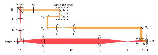
**Fig. 2** A schematic of the interferometer with a Mach–Zehnder off-axis digital holography configuration. The camera is on the Fourier plane. Optical sections are reconstructed using a 2-D spatial Fourier transform. ND, neutral density filter;  $L_1 - L_7$ , lenses;  $BS_1 - BS_3$ , beam splitters;  $M_1 - M_5$ , mirrors; FP, Fourier plane; IP, image plane;  $f_5 = f_6 = 150$  mm;  $f_7 = 50$  mm. The translation stage defines the coherence gate for time-domain ranging.
