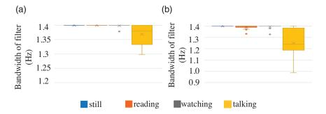
**Fig. 15** Change in adaptive filter bandwidth for different scenarios: the range of motion increases from still task to talking. With an increase of motion, the motion interference component in the iPPG signal increases and the bandwidth of the bandpass filter is the largest for the still task and smallest for talking task.
