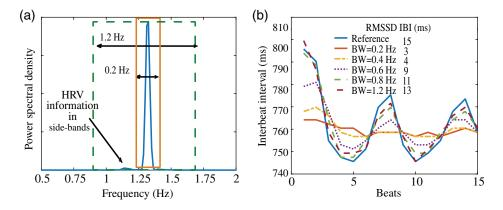
**Fig. 2** (b) On using a large BW and including the information in the sidebands of the fundamental harmonic, the estimates of HRV RMSSD are more accurate and follow ground truth more closely. (a) HRV information is in the sidebands of the fundamental harmonic because of quasi-periodicity of pulse signal.
