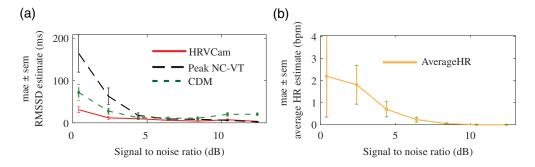
**Fig. 12** (a) Distribution of mae in RMSSD across different SNR obtained from iPPG signal computed for different activities. For lower SNR [calculated with Eq. (24)] videos, HRVCam shows large improvements. (b) Distribution of error in average heart rate across SNR
