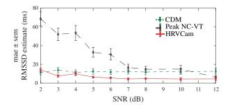
**Fig. 14** The SNR of the cPPG signal degrades on increasing the power of additive white noise added to the signal. The performance of peak-based approach (Peak NC-VT) deteriorates at a faster rate than frequency-based approaches (HRVCam and CDM).
