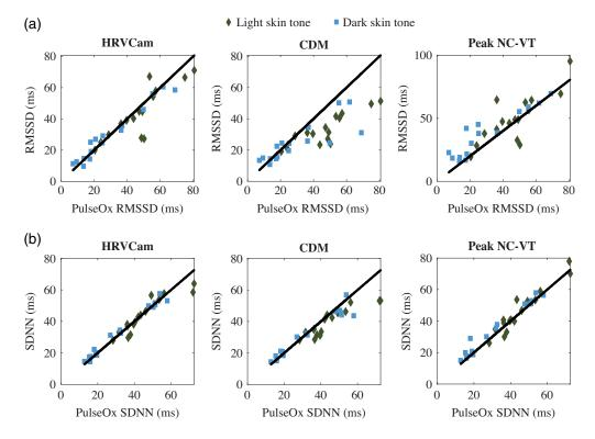
**Fig. 6** Scatterplot comparison of HRV metrics (a) RMSSD and (b) SDNN derived from iPPG with HRVCam, CDM, and Peak NC-VT methods, respectively, against ground truth pulse oximeter for different skin tones. Note that different *y* axis scales are used for the methods to accommodate all the points).
