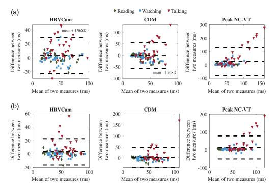
**Fig. 10** Bland–Altman plot of HRV metrics (a) RMSSD and (b) SDNN derived from iPPG with HRVCam, CDM, and Peak NC-VT methods, respectively, against ground truth pulse oximeter for different motion scenarios.
