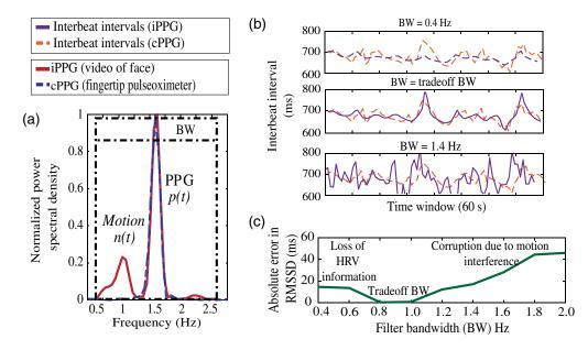
**Fig. 1** (a) Comparison of the normalized power spectral density of the video iPPG signal and the ground truth cPPG signal. (b) IBI estimates from iPPG compared with the ground truth for different BWs. The estimates are most accurate for the BW of 1 Hz (middle figure). (c) Trade-off between losing HRV information and rejecting motion interference by comparing the error in RMSSD estimate across different BWs.
