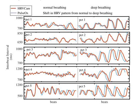
**Fig. 13** Change in HRV pattern from normal breathing to deep breathing in a participant: In the left panel, the pattern of IBI is random while the person breathes normally, and its HRV variability is lower. On the right panel, during deep breathing due to respiration sinus arrhythmia, the pattern of the IBI is sinusoidal syncing with the respiration, and HRV variability increases. We show examples of five random participants (top to down).
