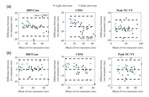
Fig. 7 Bland–Altman plot of HRV metrics (a) RMSSD and (b) SDNN derived from iPPG with HRVCam, CDM, and Peak NC-VT methods, respectively, against ground truth pulse oximeter for different skin tones.
