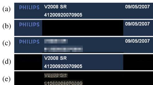
**Fig. 3** Closeup views of original and redacted text. (a) Original. (b) Decompressed, redacted, recompressed (with identity quantization tables). (c) Selective block redaction. (d) Difference original versus recompressed. (e) Difference original versus selective block redaction.
