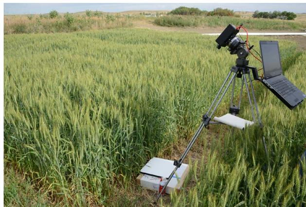
**Fig. 1** The hyperspectral imager scanning across the three kochia biotypes (susceptible, glyphosate-resistant, and dicamba-resistant) in a field of wheat at the SARC in Huntley, Montana, on July 6, 2016. The white panel is our Spectralon calibration panel used for all calibration measurements in this study.
