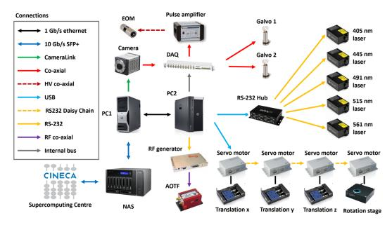
**Fig. 4** Schematic view of the hardware architecture of the microscope. Different kinds of physical connections are depicted with different colors.
