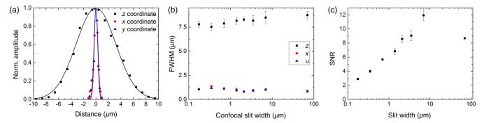
**Fig. 3** Optical characterization. (a) Exemplary lateral and axial intensity profiles of nanometric beads and fits to Gaussian curves. (b) Full-width at half-maximum (FWHM) of the Gaussian fits with confocal slit width. Each data point is the average of 10 bead profiles. (c) Signal-to-noise ratio (SNR) as a function of slit width.
