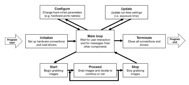
Fig. 9 Schematic view of the work flow of a representative Murmex component operating a camera.
