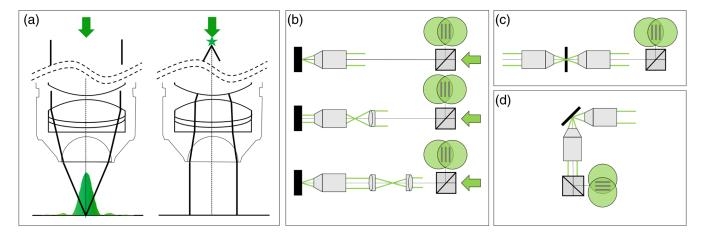
**Fig. 8** (a) Working principle of a microscope objective (left): a collimated input beam is converted into a spherical wavefront. Right: inverted light path, a focal spot in the back aperture creates a collimated output. (b) Recursive placement of lenses using the sample mirror in back-reflection mode, (c) in transmission mode, and (d) in reflection mode.
