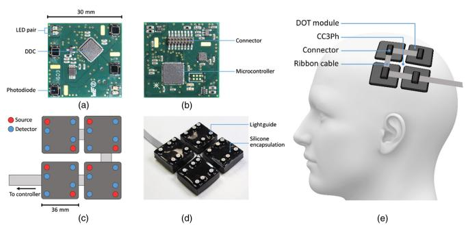
**Fig. 4** The modular DOT system described by Chitnis et al. The front and rear views of the modular PCB are shown in (a) and (b), respectively. The  $2 \times 2$  grid pattern of the system is shown in (c), and the encapsulated system is shown in (d). (e) Demonstrates how this four-module system was arranged on the scalp. This figure is taken and modified with permission from Ref. 37.
