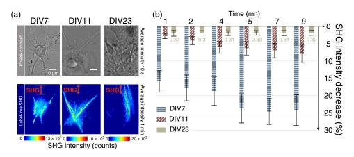
**Fig. 4** Nocodazole-induced SH intensity depletion from the cytoskeleton of neurons at different stages of maturity. (a) Top panels: PC images of cultured neurons at different stage of maturity. Bottom panels: respective label-free SH images averaged over 10 s during the control conditions. (b) Histograms of SH intensity decreases (in percentage) as a function of the time of exposure to a  $10-\mu$ g/ml solution of nocodazole.
