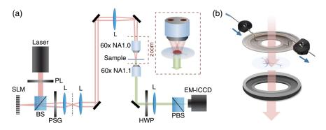
**Fig. 1** Imaging configuration. (a) Schematic representation of the SH microscope, with optical components: SLM, polarizer (PL), beam splitter (BS), polarization state generator (PSG), achromatic lens (L), dichroic beam splitter (DB), NA, HWP, and polarizing BS (PBS). (b) Layout of the sample holder, with bottomed culture coverslips inserted in a low-profile, open bath chamber from Warner Instruments (Series 40 Quick Change Imaging Chambers RC-40LP).
