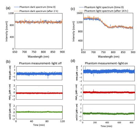
**Fig. 6** Phantom measurements in dark and light showing the stability of the miniCYRIL system. (a) and (b) The spectral data and concentration changes in a tissue-like phantom ( $\mu a = 0.02$  and  $\mu' s = 0.9$ , [mm<sup>-1</sup> mol<sup>-1</sup>]) for 2 h when the shutter of the light source is closed. (c) and (d) The spectral data and concentration measurements for 14 h, when the same phantom is illuminated (shutter open). Integration time for both measurements is 1 s and SDS is 4 cm.
