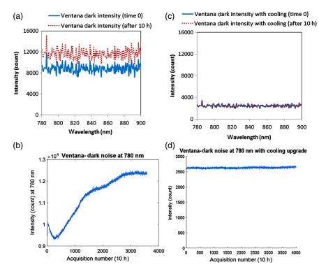
**Fig. 5** (a) Dark intensity spectrum measured across 780 to 900 nm every 10 s when the slit of the spectrometer is closed at time 0 and after 10 h. (b) The dark intensity changes at wavelength 780 nm over 10 h. (c) Dark intensity spectrum measured across 780 to 900 nm every 10 s with the upgraded unit, the slit is closed at time 0 and after 10 h. (d) The dark intensity changes at wavelength 780 nm over 10 h.
