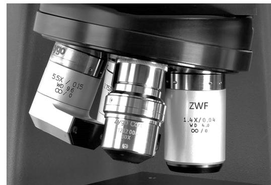
**Fig. 4** The 1.4× interferometer (to the right in the figure) mounted on a turret with parfocal 2.75× and 5.5× Michelson objectives and a 20× Mirau objective. These lenses all have the same 60-mm parfocal distance.
