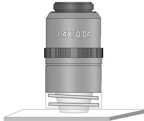
**Fig. 3** Compact 1.4× interference objective based on a 144-mm focal length microscope objective and the configuration of Fig. 2.
