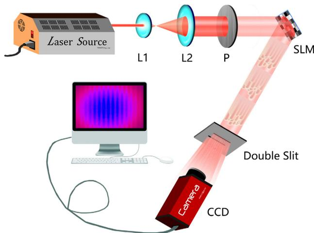
**Fig. 3** Experimental setup of generation of partially coherent beams. L1 and L2, lens; P, polarizer; SLM, spatial light modulator.
