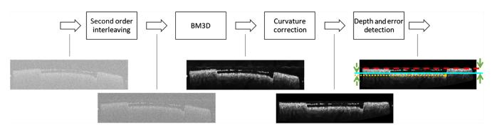
Fig. 4 To obtain the final image and metrics for analysis, a series of image processing steps are performed, including second-order interleaving, BMD3 filter, curvature correction, and depth/error detection.
