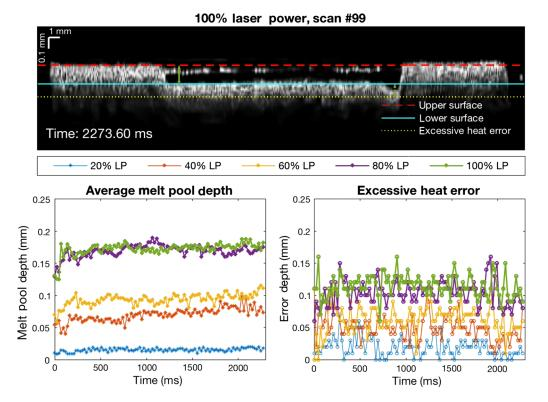
Fig. 5 OCT imaging after sintering reveals a slight upward trend in average melt pool depth with time as the heat diffuses through the powder bed. Also, increasing laser powers create deeper melt pools and larger excessive heat errors on the temporally distal end of the sintering laser sweep (right side) (Video 1, MP4, 23.6 MB [URL: https://doi.org/10.1117/1.OE.57.4.041407.1]).
