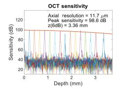
Fig. 2 The OCT system was experimentally determined to have a peak sensitivity of 98.6 dB and an axial resolution of 11.7  $\mu$ m. By fitting a Gaussian curve to the peak sensitivities at increasing pathlengths, the imaging range (6 dB) was calculated to be 3.36 mm.
