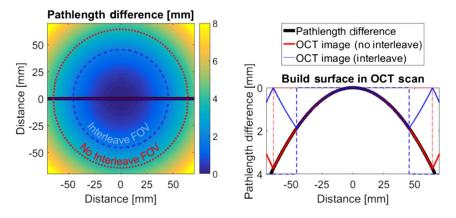
Fig. 6 The imaging range of the OCT system limits the FOV because postobjective scanning hyperbolically varies the path length difference between the flat powder surface and the static reference arm mirror. The FOV and cross-sectional image with no interleaving is pictured by the red lines. The FOV is smaller after interleaving (blue), and the corresponding cross-sectional image exhibits faster aliasing due to down sampling in the k-space domain.
