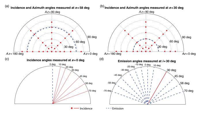
Fig. 3 Schematic showing the multiple measurement geometries acquired with the incidence angle indicated in red and the emission angle indicated in blue. Out-of-plane phase angle measurement geometries are shown in (a) and (b) where the emission angle is fixed and the incidence and azimuth angle vary. (c) and (d) The in-plane measurement geometries.
