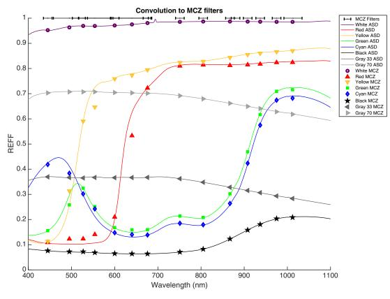
Fig. 8 Convolution of spectra on calibration target materials to MCZ filter set.
