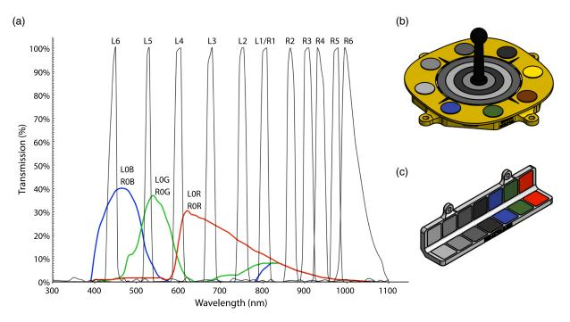
**Fig. 1** (a) Preliminary estimates of MCZ filter transmission profiles. (b) Schematic of MCZ primary calibration target. Not shown, below each of the eight circular color and grayscale patches around the periphery lies a strong circular sweep magnet intended to minimize accumulation of Martian dust on the central part of these circular patches. (c) Secondary calibration target schematic.
