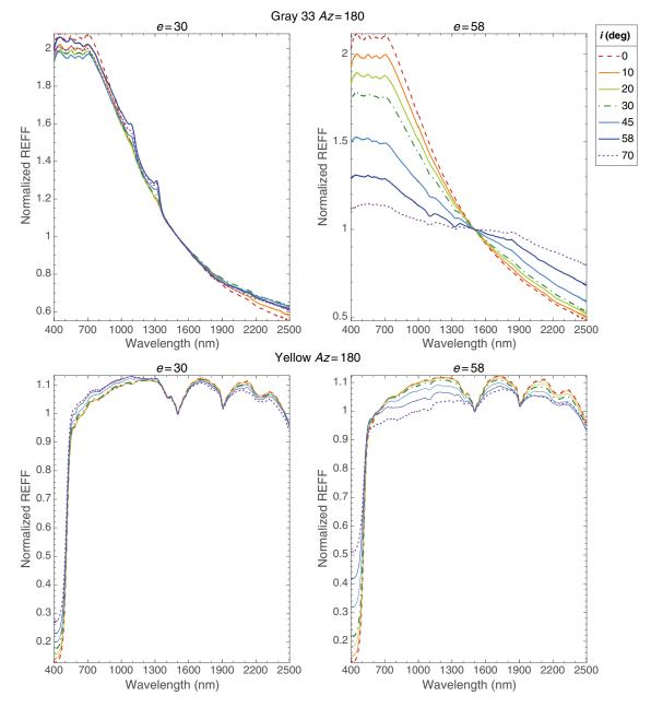
**Fig. 9** Slope as a function of viewing geometry for the same set of measurements for gray 33 and yellow samples at Az = 180, normalized to REFF at 1500 nm. (left) MCZ relevant wavelengths, (right) full wavelength range, (top) Gray 33, and (bottom) Yellow.
