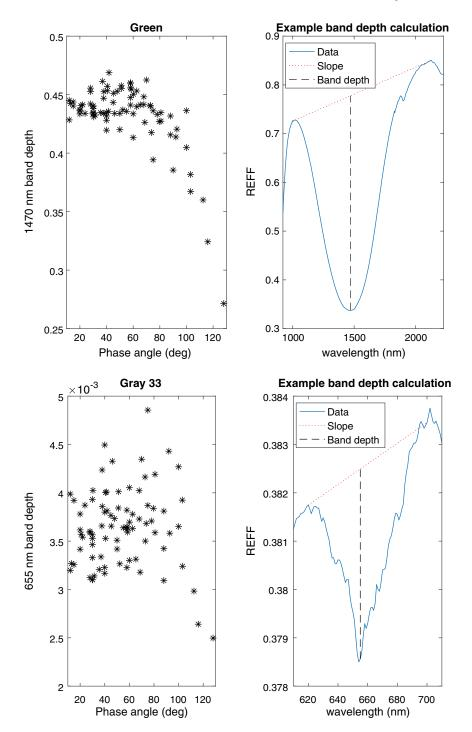
Fig. 10 Band depth calculations and changes with phase angle. (left) Band depths at all phase angles, (right) Example band depth calculation, (top) Green 1470 nm absorption, and (bottom) Gray 33 655 nm absorption.
