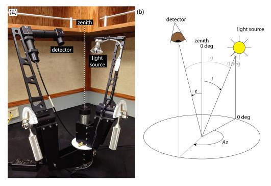
**Fig. 2** (a) Goniometer set up at the Caltech Earth and Planetary Remote Sensing Laboratory. A fiber optic cable from the spectrometer is fed into the detector assembly. (b) Measurement convention used in this study. Arrows point in positive degree direction.
