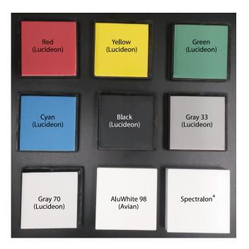
**Fig. 4** Calibration targets used in this study with manufacturer indicated in parentheses and Spectralon<sup>®</sup> for comparison. All of the Lucideon targets are mounted on a black plastic holder. The white target is not mounted.
