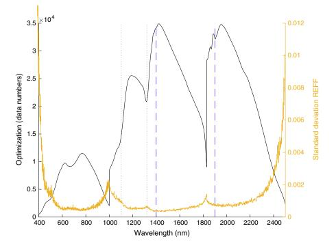
Fig. 5 Optimized instrument response for the three detectors of the ASD FieldSpec 3<sup>®</sup> exhibiting features at 1100 and 1320 (dotted gray lines) that should be interpreted as measurement artifacts and 1400 and 1900 nm from water (dashed blue lines) that should be interpreted with caution. Incidence angle was 12 deg and emission angle 0 deg. Standard deviation REFF for 100 successive Spectralon<sup>®</sup> measurements are shown in orange with corresponding right axis.
