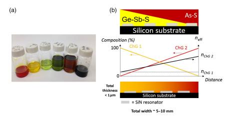
**Fig. 8** (a) Multiple solutions of various ChG materials<sup>88</sup> dissolved in amine solvents. (b) (top) Bilayer design of a GeSbS and AsS gradient profile and (bottom) actual effective index profile of the measured gradient layer, as a function of position across a SiN resonator array. (b) Reproduced with permission from Ref. 56. Copyright 2017 ACS Publications.
