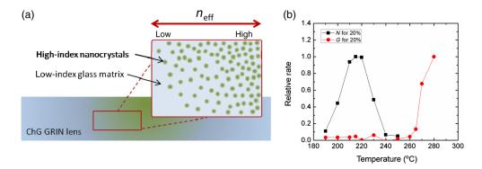
**Fig. 4** (a) ChG GRIN lens where a gradient index is created through the spatial control of high refractive index particles embedded in a lower refractive index glass matrix. (b) The nucleation (*N*) and growth-like (*G*) rates for GAP-Se glasses with 20 mol. % PbSe. (a) Reproduced with permission from Ref. 42. Copyright 2016 SPIE. (b) Reproduced with permission from Ref. 46. Copyright 2019 Wiley.
