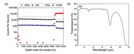
**Fig. 2** (a) SIMS profile of the compositional variation induced by thermal poling. The signal decrease of Ge, Sb, and S at  $\lambda=6.5~\mu\mathrm{m}$  is due to charging of the sample during the measurement, but illustrates the near-surface depletion of Na after poling. (b) Transmission spectrum (not corrected for Fresnel loss); sample thickness = 1.04 mm and sample diameter = 10 mm (as shown in Fig. 1). (a) Reproduced with permission from Ref. 38. Copyright 2018 OSA.
