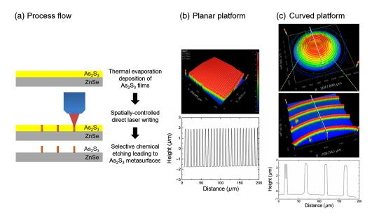
**Fig. 11** (a) A schematic of two-step photochemical process flow where large area, laser-written metasurface structures are realized via selective chemical etching. (b) A demonstration of a large area, high fidelity grid structures (7.5- $\mu$ m grid spacing) on a planar platform. (c) A demonstration of laser written and etched circular ring patterns on a curved IR lens platform.
