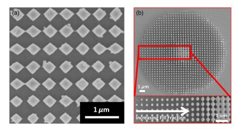
**Fig. 12** (a) Ge-containing As-Se film array pattern  $[Ge_5(As_{40}Se_{60})_{95}]$  after t=4 years of aging. Features show minor deterioration at their edges but retain their as-written lateral dimensions. (b) An  $As_2S_3$  meta-lens created using MPL. (a) and (b) Reproduced with permission from Ref. 111. Copyright 2018 OSA.
