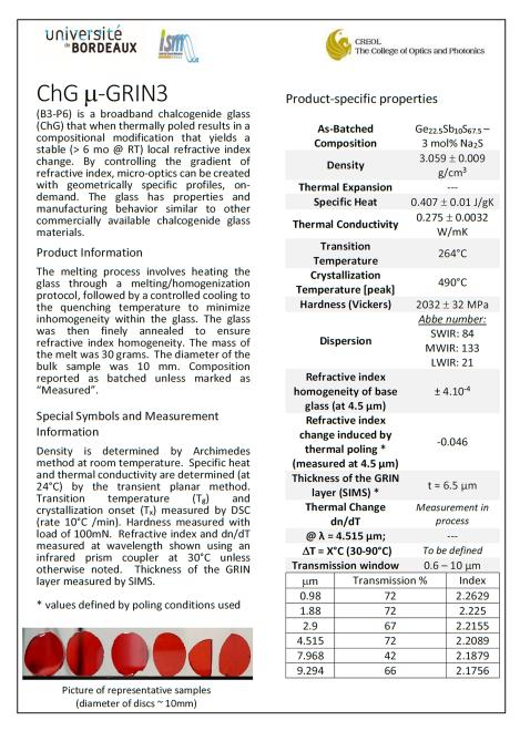
**Fig. 1** Sample specification sheet for ChG  $\mu$ -GRIN3 GeSbS (3 mol. % Na<sub>2</sub>S) glass summarizing characteristic material properties of the unpoled materials. Such data are critical to optical designers examining the potential of the candidate materials in their system designs.
