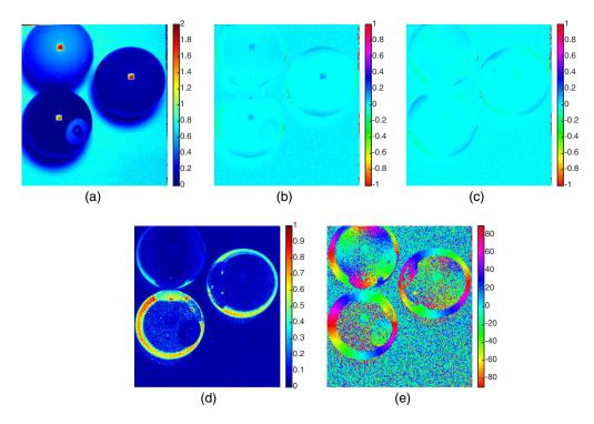
**Fig. 6** (a)–(c) Stokes components  $S_{0,s}$ ,  $S_{1,s}$ , and  $S_{2,s}$  for spectral band  $s = G_{bg}$ . (d)–(e) DOLP<sub>s</sub> and AOLP<sub>s</sub> for spectral channel  $s = G_{bg}$ .
