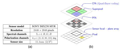
**Fig. 1** The color PFA (CPFA) sensor: (a) sensor characteristics and (b) spatial arrangement of the SONY IMX250 MYR sensor. Each pixel is covered by one linear polarization filter and one spectral filter.
