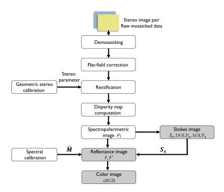
Fig. 3 Practical imaging pipeline.
