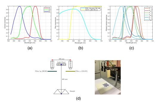
**Fig. 2** (a) The CPFA camera spectral sensitivities (only the 0-deg polarization channel is shown because the four polarization channels are very similar). The sensitivity is obtained by characterizing the sensor with a spectral resolution of 10 nm from 370 to 750 nm. (b) Spectral transmission of the bandpass filters provided by the manufacturer. (c) Total spectral sensitivities of the cameras after combination. (d) Setup configuration.
