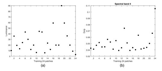
Fig. 5 (a) Luminance and (b)  $\text{DOLP}_{G_v}$  plot of the 24 MCCPP training samples.
