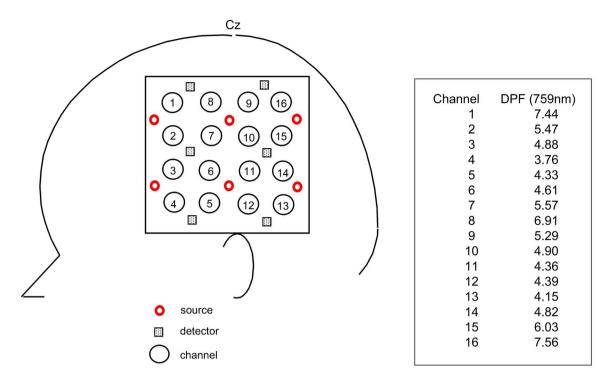
Fig. 4 Different path length factors measured on the left scalp adjacent to the somatosensorimotor cortex in a 23-year-old healthy adult. The wavelength is 759 nm.
