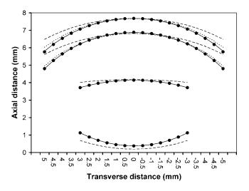
**Fig. 1** Profiles and axial separations of actual surfaces (solid lines) compared to uncorrected measured surfaces (dashed lines) and those corrected using built in AS-OCT software (dashed lines) and the equations shown in Tables 1 and 2 (circles). Each profile represents the average of the five model eyes tested.
