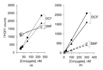
**Fig. 3** (a) Comparison of TPOFF measurement of standard solutions of G5-6T (triangle symbols) and G5-6T-FA (square symbols) using SMF and DCF probes. The TPOFF photocounts of different concentrations of the standard solutions are measured by inserting the fiber into the solution. The data shown are the mean  $\pm$  SE of four to five such counts taken for each concentration of the standard. (b) Data corrected for the detection background.
