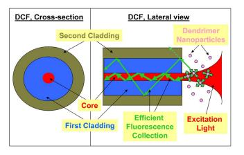
**Fig. 2** Schematic drawing of the DCF having a 10- $\mu$ m inner core, 123- $\mu$ m first cladding, and 178- $\mu$ m second cladding diameters. Unlike the SMF we have described previously, this newly developed DCF allows collection of emission fluorescence not only through the fiber core, but also through the inner cladding, resulting in increased efficiency.
