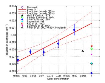
Fig. 6 Absorption coefficient of Intralipid® at 750 nm plotted against water concentration along with literature data. The dotted lines indicate 95% confidence interval for the linear fit.
