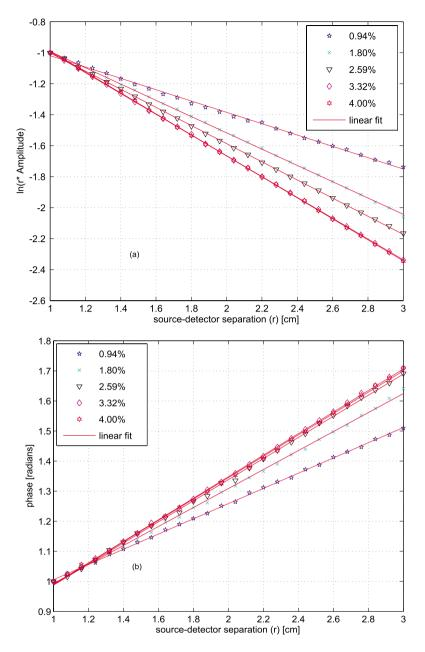
Fig. 2 (a) Logarithm of source-detector separation times normalized ac amplitude and (b) normalized phase variation versus source-detector separation at 750 nm for five Intralipid® concentrations.
