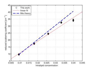
**Fig. 8** Reduced scattering coefficients at 750 nm versus Intralipid® concentration. The errorbars indicate 95% confidence intervals. The solid line is a linear fit to the experimental data. The dashed line shows the Mie theory results.
