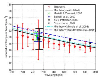
**Fig. 9** Reduced scattering coefficient (triangular markers with error bars) values for a 2% solution of Intralipid® plotted against wavelength. The solid line corresponds to the Mie theory values calculated based on our particle size measurement. Data reported at 750 nm are staggered a little to make them visible. The error bars indicate 95% confidence interval.
