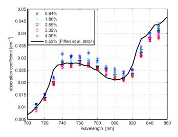
**Fig. 4** Absorption coefficient of Intralipid. Data reported by Pifferi et al.<sup>21</sup> (solid line) are included for comparison. The error bars indicate a 95% confidence interval.
