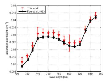
**Fig. 7** Extrapolated absorption coefficient (triangular markers with error bars) for water from Intralipid® measurements versus wavelength. The solid curve represents water absorption data reported by Kou et al.<sup>28</sup> The error bars correspond to ±2 standard deviations.
