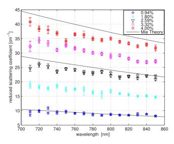
**Fig. 5** Reduced scattering coefficient of Intralipid®. The solid line corresponds to a Mie theory calculation based on our particle-size measurements. The error bars indicate a 95% confidence interval.
