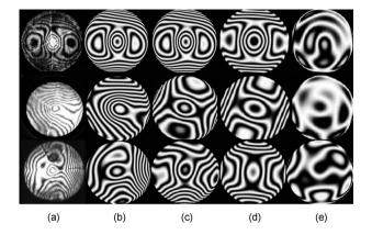
**Fig. 5** In columns: (a) Recorded interferograms for three different lenses. (b) Simulated interferograms with fit coefficients. (c) Simulated interferograms with fit coefficients excluding tilts and defocus. (d) Simulated interferograms with fit coefficients only for Zernike polynomials  $Z_{4\prime}^0$   $Z_2^{\pm 2}$  and  $Z_6^0$ . (e) Interferograms for differences between (3) and (4).
