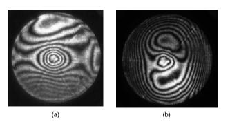
**Fig. 2** (a) Interferogram in focus (pinhole close to circle of least confusion). (b) Interferogram with some amount of defocus.
