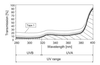
**Fig. 1** Determination of the sum transmission spectrum and the corresponding areas beneath the sum spectrum used to determine the average UVA und UVB sum transmissions (sunscreen sample 7 with SPF 16).
