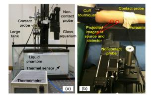
Fig. 2 Experimental setup for concurrent flow measurements using contact and noncontact probes in a liquid phantom solution (a) and a forearm muscle (b).
