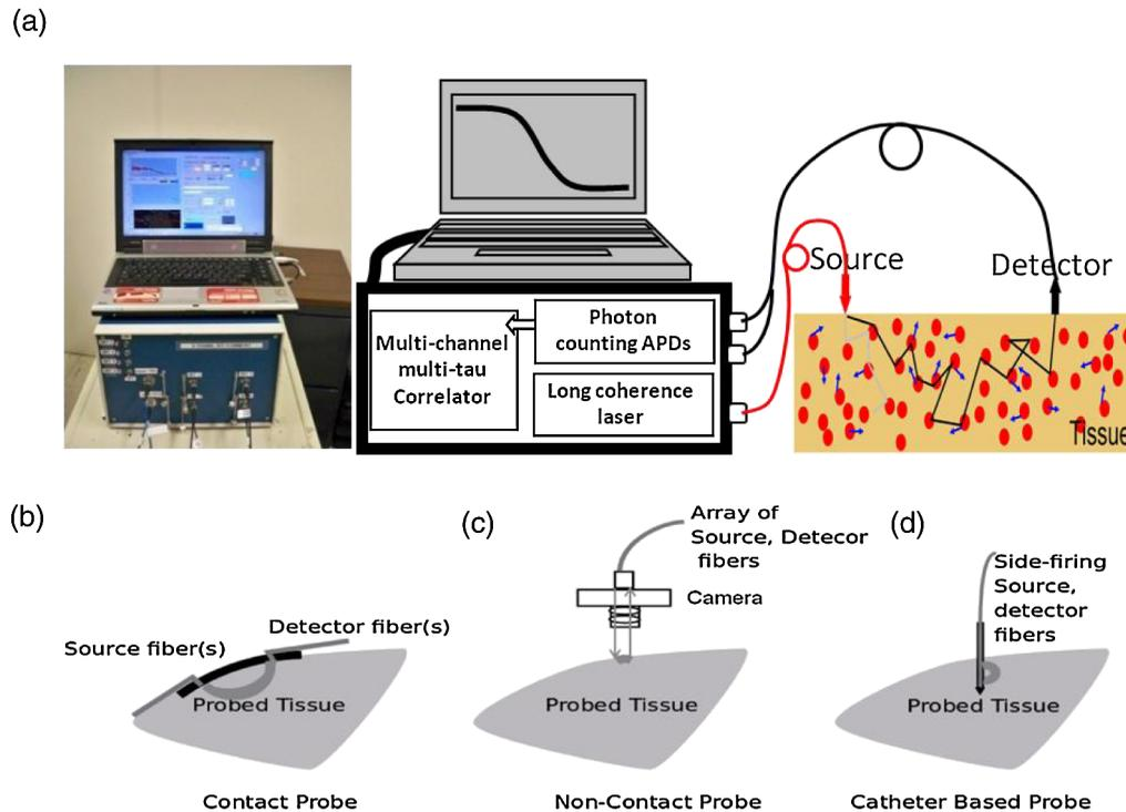
**Fig. 1** (a) Portable 4-detection-channel DCS system (dimensions: 8'' × 12'' × 18''), from left to right: instrument photo, DCS diagram, probe-tissue interface. Three examples of DCS probes: (b) contact probe, (c) noncontact probe, and (d) catheter-based probe.
