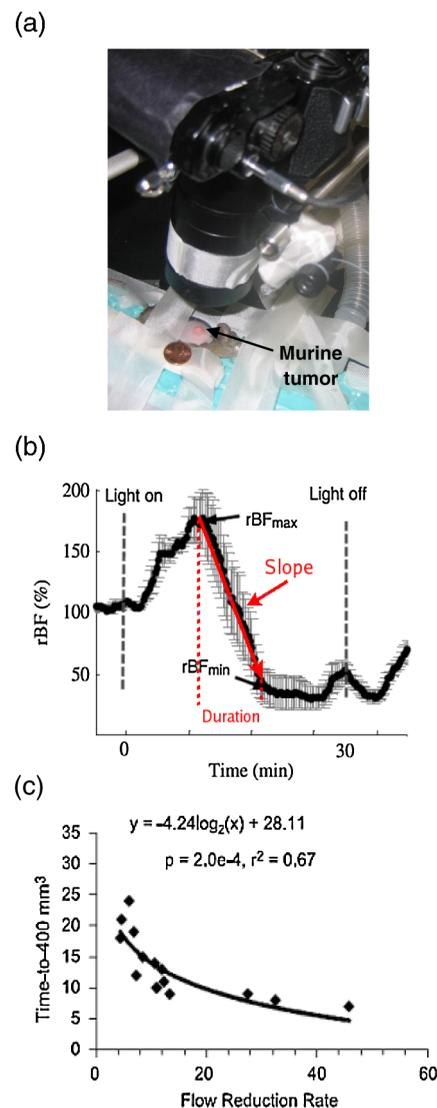
**Fig. 3** (a) Photo of noncontact camera probe, (b) representative trace of tumor blood flow (rBF) during PDT, and (c) correlation between treatment durability (time-to-400 mm<sup>3</sup>) and flow reduction rate (slope) during PDT.<sup>5</sup>
