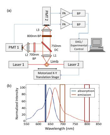
**Fig. 1** (a) Schematic of the dual channel DFFC prototype. (b) Normalized absorption (blue) and emission (red) spectra of Vybrant-DiD fluorophore. The wavelength range of the laser (blue line, 635 nm) and two emission filters (red rectangles, 700 and 800 nm) are indicated.
