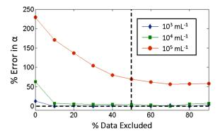
**Fig. 3** Estimation of  $\alpha$  from phantoms with (a) 10<sup>3</sup>, (b) 10<sup>4</sup> and (c) 10<sup>5</sup> microspheres/mL, respectively, with fixed fractions of data points with highest deviation from the mean removed from the calculation. The dotted line represents the selected threshold which allowed stable estimation of  $\alpha$  for sphere concentrations below 10<sup>4</sup>/mL.
