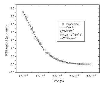
Fig. 9 PTE output recorded for flowing ink (open squares) and the best theoretical fit (dash). Pump wavelength is 589 nm.
