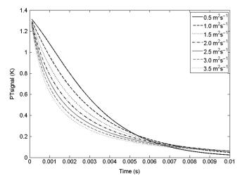
**Fig. 6** Simulated PT transient response of static blood, for excitation at 589 nm, for the diffusivity range of  $0.5 \times 10^{-7}$  to  $3.5 \times 10^{-7}$  m<sup>2</sup> s<sup>-1</sup>.
