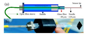
Fig. 3 (a) Architecture of the photothermal endoscope (PTE). The lowest inner needle diameter used was 120  $\mu m.$  (b) Photograph of the laboratory prototype.
