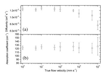
Fig. 10 Dependence of endoscopically measured diffusivity (a) and absorption coefficient (b) of the flowing ink solution on the true flow velocity.
