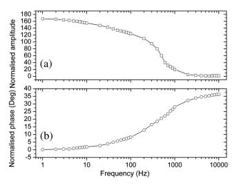
Fig. 7 Frequency response of the PTE: (a) amplitude and (b) phase. An offset correction has been applied to the phase to read 0 deg at 1 Hz.
