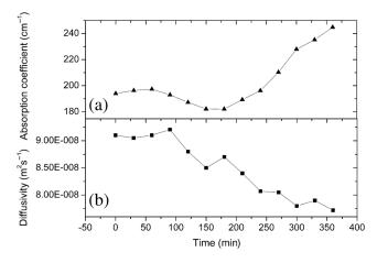
Fig. 12 Variation of (a) absorption coefficient and (b) thermal diffusivity of goat shoulder marrow with time, estimated using PTE. The bone had  $\sim$ 2-cm thick meat over it.
