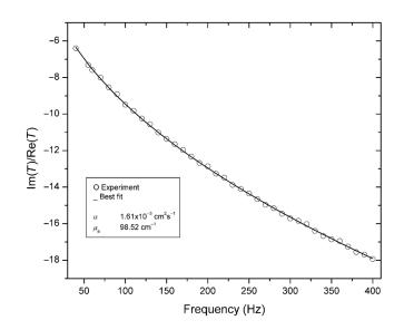
**Fig. 8** Frequency-swept Im(T)/Re(T) response (open circles) of static ink solution excited with 589-nm diode laser and the best theoretical fit (dash).
