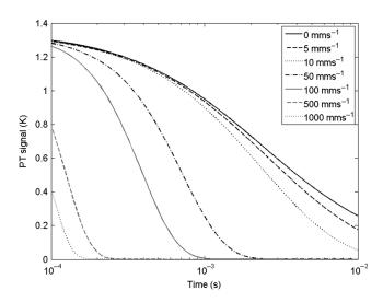
Fig. 5 Simulated PT transient response of blood, for excitation at 589 nm, for the flow velocity ranging from 0 to  $1000 \text{ mm s}^{-1}$ .
