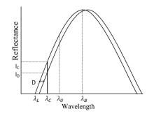
Fig. 2 Geometry of the fiber Bragg grating (FBG) reflection spectrum with the overlap of probe laser line.
