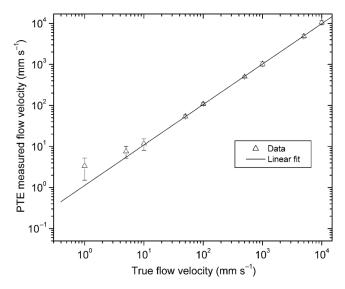
Fig. 11 Endoscopically measured flow velocity versus true velocity for the ink solution.
