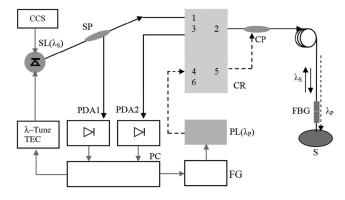
Fig. 1 Schematic of the thin photothermal (PT) endoscope.
