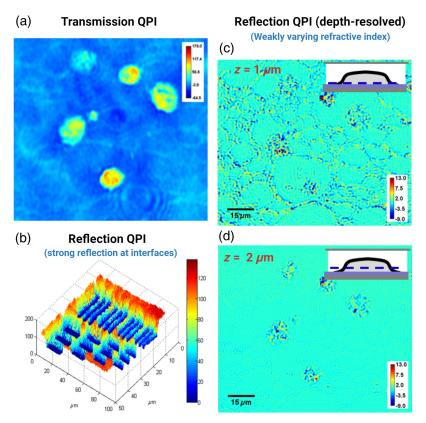
**Fig. 3** Representative images from (a) transmission QPI of cells embedded in resin-based substrates, (b) reflection QPI of a USAF target in the presence of strong interfaces, and (c) and (d) reflection QPI of weakly scattering objects (cells embedded in resin-based substrates) in the absence of strong interfaces at different depths.
