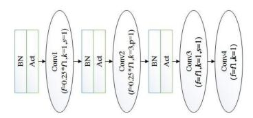
**Fig. 3** ResNet50 res\_units network architecture. f1 represents the input filter numbers, k is the kernel, s is the stride, and p is the padding.
