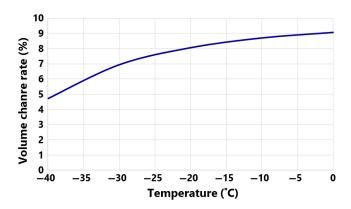
Fig. 2 Volume change rate when supercooled water is frozen.
