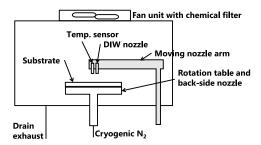
Fig. 6 An overview of the freeze-cleaning module.
