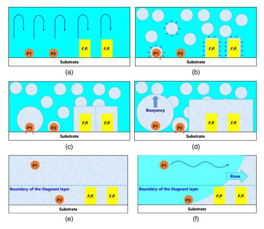
**Fig. 4** The model of freeze-cleaning method. (a) Water behavior from 4°C to before freezing begins (-38°C), (b) ice formation in the water and particle removal force by volumetric expansion, (c) ice growth by continuously cooling from the substrate, (d) escape the FC particle by buoyancy from the substrate, (e) entire water is frozen, and (f) particle only escaped from the stagnant layer is rinsed away from the substrate.
