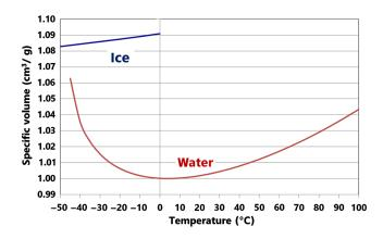
Fig. 1 Temperature dependence of the specific volume of ice and water plotted based on Refs. 15 and 16.
