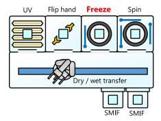
Fig. 5 Outline of MC150-plus and layout of the freeze-cleaning module.
