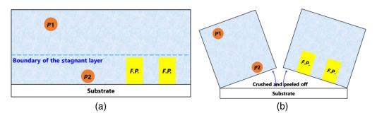
**Fig. 11** Model of the long freezing duration and the subsequent ice crushing. (a) After the entire water is frozen [same as Fig. 4(e)] and (b) additional cooling causes the ice crush along with everything peeling from the substrate.
