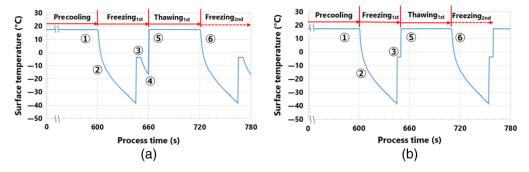
**Fig. 7** Substrate surface temperature with respect to the process using cryogenic  $N_2$  on the underside of the substrate. (a) The thawing step begins after the temperature decreases for the second time in the freezing step. This corresponds to Fig. 4(f). (b) The thawing step begins when the temperature is maintained at  $-4^{\circ}$ C in the freezing step. This corresponds to Fig. 4(d).
