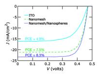
Fig. 2 J - V characteristics of c-Si solar cells with different frontside structures.
