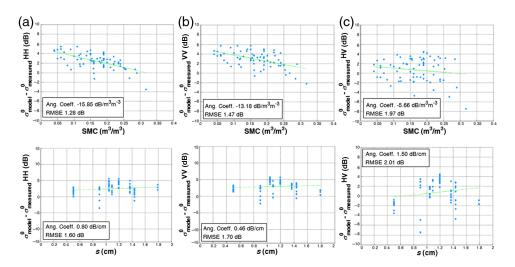
**Fig. 3** Difference between the backscattering coefficient simulated by the Oh and Sarabandi model and the measured ones for (a) HH, (b) VV, and (c) HV polarizations. The upper figures show the error as a function of soil moisture and the lower ones as a function of soil roughness. The green line represents the best fitting line, and its slope and RMSE are reported in the legend.
