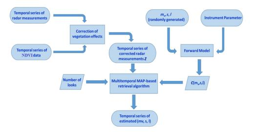
Fig. 1 Processing chain of the MLTA.
