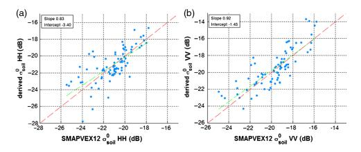
**Fig. 12** Comparison between the backscatter coefficients of the soil backscattering contributions provided by the *in situ* measurements, using the modified Oh and Sarabandi model, and that derived from the radar measurements using the adopted empirical model for RRI. Dashed red and green lines represent the perfect agreement and the best fitting lines, respectively. The slope and the intercept values of the best fitting line are reported in the legend.
