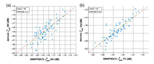
**Fig. 15** Comparison between the backscatter coefficients of the soil backscattering contributions provided by the in situ measurements, using the modified Oh and Sarabandi model, and that derived from the radar measurements using the adopted empirical model for RRI over corn crops. Dashed red and green lines represent the perfect agreement and the best fitting lines, respectively. The slope and the intercept values of the best fitting line are reported in the legend.
