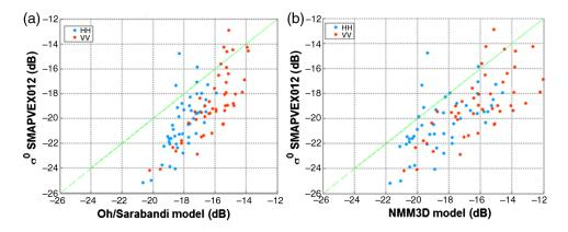
**Fig. 2** Comparison between modeled and measured backscattering coefficient for HH (cyan dots) and VV (red dots) polarizations. (a) and (b) refer to the Oh and Sarabandi and NMM3D simulations. Green line represents the perfect alignment.
