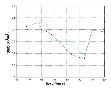
**Fig. 7** Temporal trend of soil moisture retrieved by MLTA (green line) and that measured by *in situ* probes provided by the SMAPVEX12 campaign (blue line) for the wheat field number 31.
