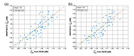
**Fig. 6** Comparison between the measured soil backscattering and those obtained through the WCM over wheat fields. Dashed red and green lines represent the perfect agreement and the best fitting line, respectively. The slope and the intercept values of the best fitting line are reported in the legend. (a) HH and (b) VV polarizations.
