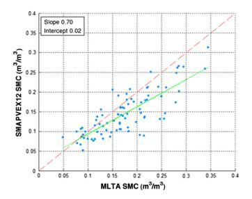
**Fig. 16** Comparison between the retrieved and *in situ* measured soil moisture over corn fields. Dashed red and green lines represent the perfect agreement and the best fitting line, respectively. The slope and the intercept values of the best fitting line are reported in the legend.
