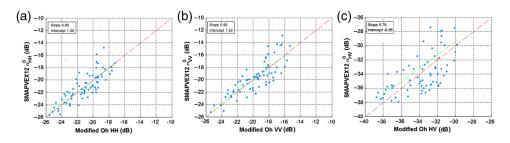
**Fig. 4** Comparison between the measured backscattering coefficient and modeled ones (derived from the LOO analysis) using the modified Oh and Sarabandi model. (a) HH, (b) VV, and (c) HV polarizations. The green line represents the best fitting line, and its slope and intercept values are reported in the legend.
