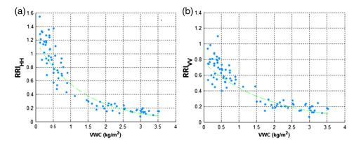
**Fig. 14** Ratio between the soil backscatter predicted from ground data using the corrected Oh and Sarabandi model, and the corn measured backscattering as a function of the VWC measurements *in situ.* (a) HH and (b) VV polarizations.
