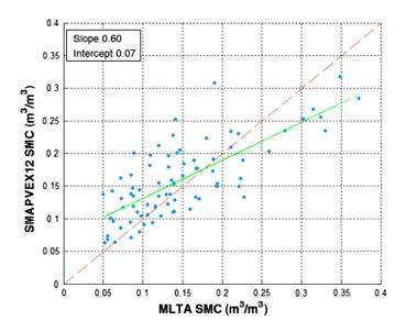
**Fig. 13** Comparison between the retrieved and *in situ* measured soil moisture over soybean crops. Dashed red and green lines represent the perfect agreement and the best fitting lines, respectively. The slope and the intercept values of the best fitting line are reported in the legend.
