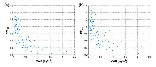
**Fig. 10** Ratio between the soil, predicted from ground data using the corrected Oh and Sarabandi model, and the soybean measured backscattering as a function of the VWC measurements *in situ*. (a) HH and (b) VV polarizations.
